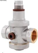
Body in dezincification resistant brass. Adjustable outlet pressure: between 1 to 5.5 bar (up to 1") or 1 to 6 bar (1.1/4" onwards). Factory setting 4 bar.
