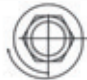
Only 3/4 Turn from Finger Tight is necessary to seal and will result in additional remakes of the fitting
